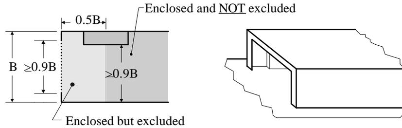
(2) **Restricted End Opening** If, because of any arrangement (except convergence of the outside plating as shown *below*), the breadth of the space is less than 90 percent of the breadth of the *deck structure at deck level*, only the space between the line of the opening and a parallel line drawn through the point where the athwartship breadth of the space is equal to 90 percent or less of the breadth of the *deck structure at deck level* is excluded.
