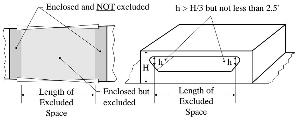
If the opening is only on one side of the *deck* structure, or the space inboard of the opening is bounded by an interior bulkhead or bulkheads, the space to be excluded is limited inboard from the opening to a maximum of one-half the breadth of the deck in way of the opening.
