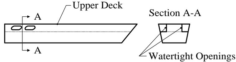
For a vessel having openings in the side of the vessel below the uppermost continuous (or “complete”) deck, which are not closed but limited inboard by weathertight versus watertight bulkheads and decks, the deck below such openings should be considered the upper deck.
