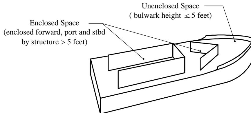
*In the situation where only a portion of a bulkhead or partition exceeds 5 feet (1.5 meters) in height, the entire inboard space in way of that portion of the structure from the deck to the top of the structure must be included in the total volume of all enclosed spaces (V).*
