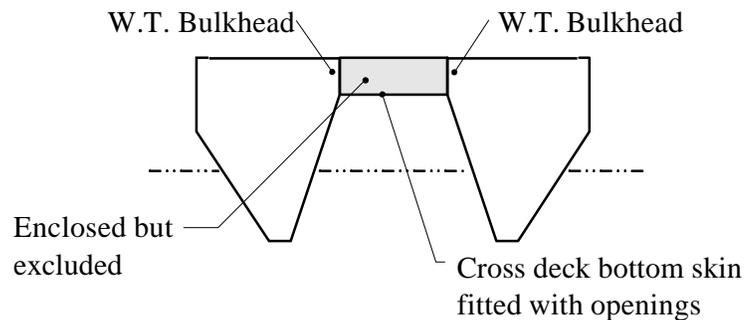
Hawse pipes, sea valve recesses, thruster tunnels, stern chutes in fishing vessels, and dredging wells in dredgers are generally treated as spaces open to the sea. Accordingly, they may be eligible for treatment as excluded spaces.
