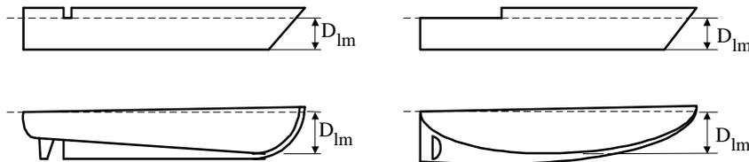
**LINE OF THE UPPER DECK** means a longitudinal line at the underside of the upper deck or, if that deck is stepped, the longitudinal line of the underside of the lowest portion of that deck parallel with the upper portions of that deck. *Discontinuities in the upper deck that do not extend from side to side of the vessel, are one meter or less in length, or are outside the boundaries of "registered length," are ignored when establishing the line of the upper deck.*
