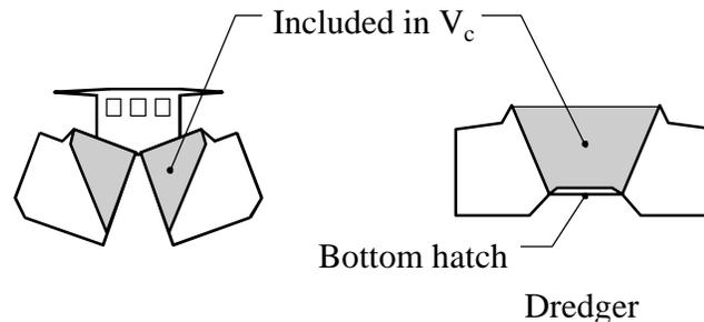
(11) **Hoppers on Deck Barges** Cargo spaces within a hopper or similar structure on deck barges. Note that under the provisions of Section 69.59, these spaces should be ignored from volume calculations if the height of the hopper above the deck does not exceed 5 feet (1.5 meters).
