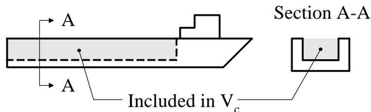
(10) **Cargo Spaces Temporarily Open to the Sea** Cargo spaces within the hulls of vessels such as split-hull barges and dredgers that are open to sea when cargo is discharged.
